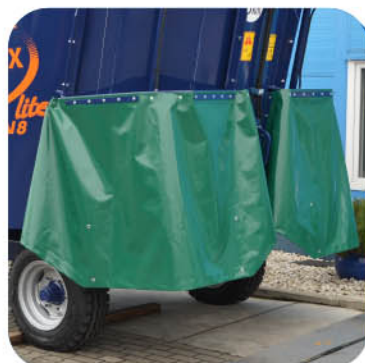
rear corner discharge
