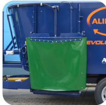
front side discharge doors
